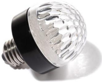
If you want to experiment, check out ( [www.superbrightleds.com](http://www.superbrightleds.com) ). An under \$10 multimeter that measures voltage, ohms of resistance and amps of current would be very helpful. The short lead and flat side of the LED is negative. Use a resistor to get a 3.6~4.2 DC voltage drop across the LED. LEDs will last for years at 20 milliamperes (0.020 amps). At 100 milliamps, their lifetime is only 100 hours.
